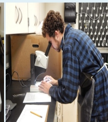
Fig. F. Todd Drake, finding micro-plastics by use of microscopes, extracting them from the Petri dish and categorizing them based on their color and shape in a chart.
