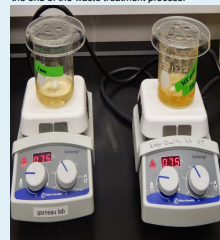
Fig. E. Sieve samples put into two beakers (1 mm and 355 \mu m combined). H_2O_2 and Fe 3+ added and heated at 75°C. While stirring on hot plates.
